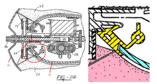
70. The colours only highlight what is already shown by the hatching. The part coloured in yellow appears to be an element that supports and holds the inner rigid wall 20, coloured in blue. The rigid wall 20 is not contacted by the medication reservoir 24, coloured in pink. The same is shown in the upper part of Fig. 11A.
