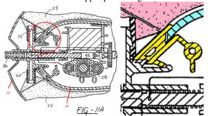
71. It is evident that Fig. 11A shows an empty gap between the medication reservoir 24 and the rigid structure 20, 26.
