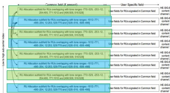
Figure 27-31—HE-SIG-B content channels and their duplication in a 160 MHz PPDU
